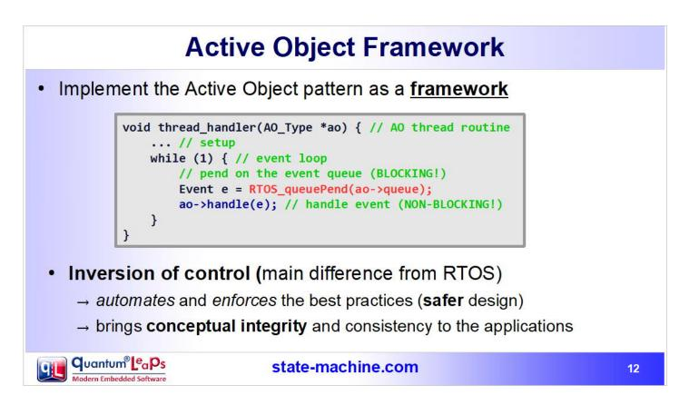
In an earlier slide, you saw how to implement the Active Object pattern manually on top of a conventional RTOS. But an even better way is to implement this pattern as a software **framework**, because a framework is the best known method to capture and reuse a software **architecture**.
