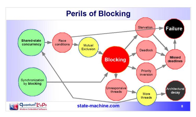
Multiple, dedicated threads are great and bring a quantum leap of improvement compared to a kitchen-sink "superloop", but the problems begin when the threads need to synchronize and communicate with each other.
