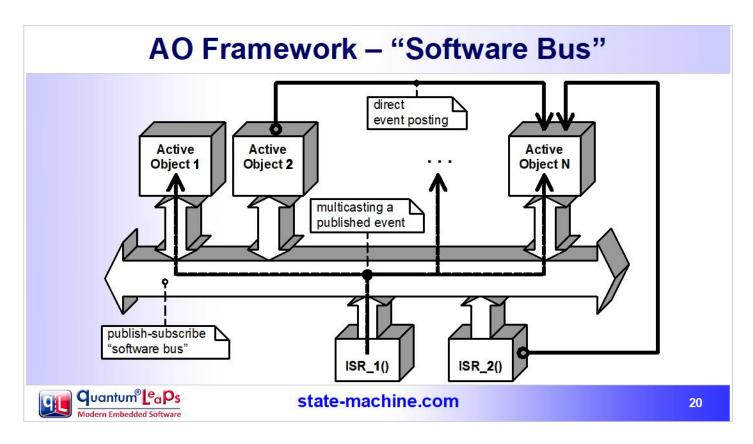
Even though an AO framework can be smaller than a conventional blocking RTOS kernel, it offers a higher level of abstraction.
