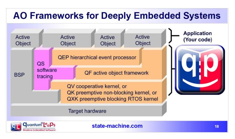
So, how do you bring it all together, in a consistent active object framework? Well, as it turns out most of such frameworks end up with a similar layered structure. Here, for example, is the structure of a minimal active object framework for RTE systems called QP:
