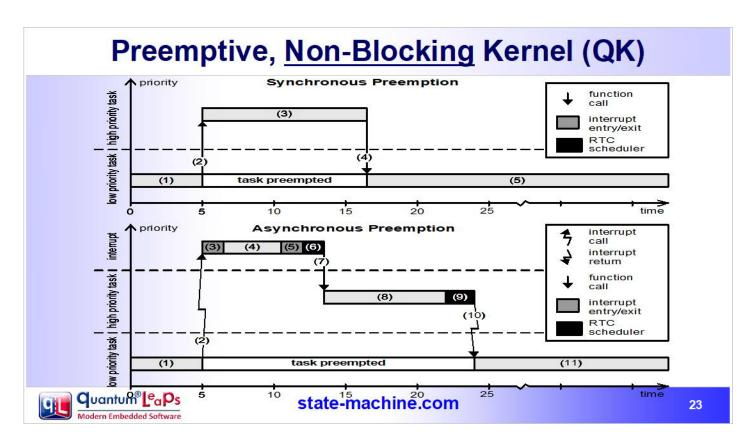
The second non-standard kernel provided in QP is really interesting. It is a very efficient, **preemptive**, priority-based, **non-blocking** kernel called QK. This kernel does not allow threads to block in the middle of run-to-completion step, but allows them to **preempt** each other (such threads are classified as "basic threads" in the OSEK/VDX terminology). The non-blocking limitation is irrelevant for event-driven active objects, where blocking is not needed anyway.
