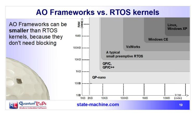
In the resource-constrained embedded systems, the biggest concern has always been about the size and efficiency of Active Object (Actor) frameworks, especially that commercial frameworks of this type accompanying various modeling tools have traditionally been built on top of a conventional RTOS, which adds memory footprint and CPU overhead to the final solution.
