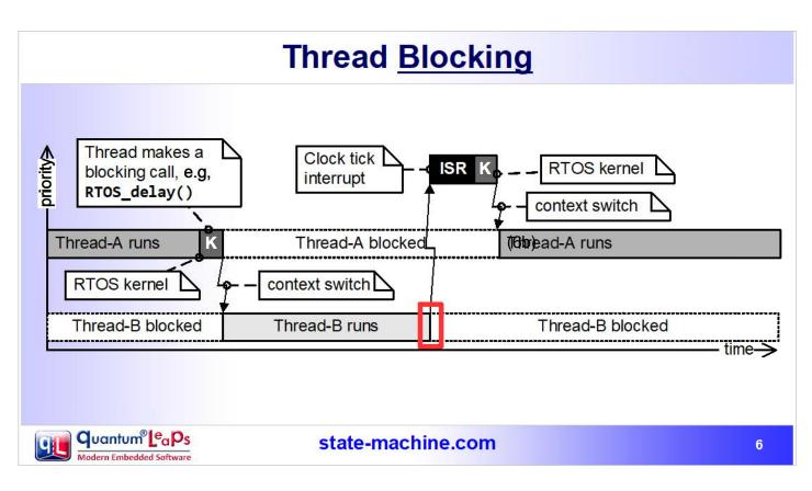
For example, a call to RTOS\_delay() from Thread-A results in a context switch to Thread-B.
