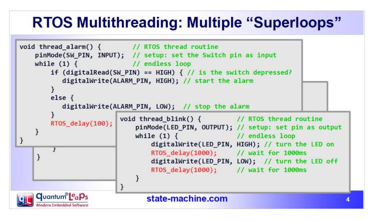
An obvious solution to the unresponsiveness of a single superloop is to allow multiple superloops to run on the same CPU. Multiple superloops can wait for multiple events in parallel.
